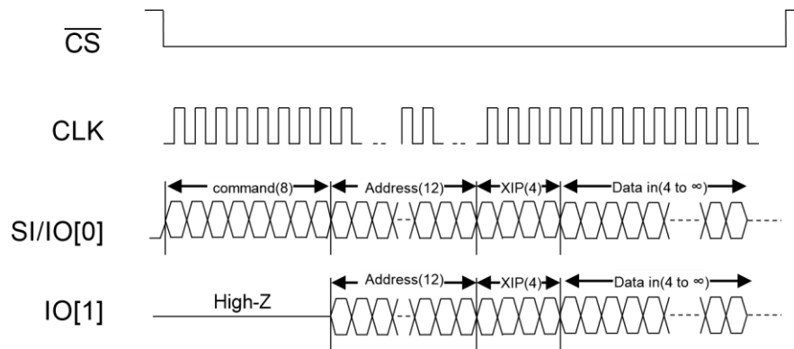
Figure 38 : Timing Description of 1-2-2 Instruction Type (Write with XIP)
